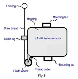
The SA-20P model is for using with the PM-11 Phytomonitor or the PTM-48M Photosynthesis Monitor. It has a 4-meter output cable with the IP67 plug at the end. The above-mentioned instruments provide necessary excitation power and the output signal processing.
