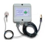
leaf temperature. The thermistor is connected to the clip by thin 0.15 mm leads to minimize heat conduction and response time. All conductors are proofed to avoid corrosion under the wet operating conditions.
